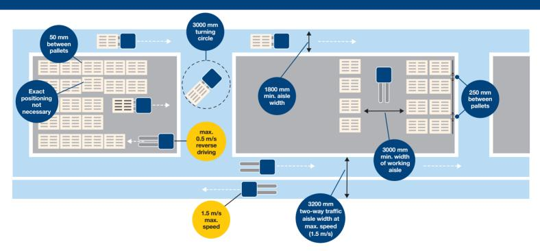
Note: Values shown are minimum space requirements in mixed traffic aisles (interaction with human workers). Actual values depend on widths of transported load and the overall customer environment.
