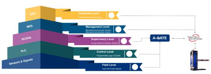
Example of the communication between the individual application levels, A-GATE, a fleet manager and the AGV/AMR.
